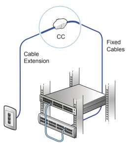
Building upon CommScope's cable engineering knowledge, the Ceiling Connector solution is designed to provide maximum performance, flexibility and durability. They feature a simplified termination that requires no special tools and can provide a high quality result in typically challenging working locations, such as over drop ceilings.
