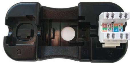
3. Present the cable at 90° to the rear of the jack and dress the wires in to the appropriate coloured IDC slots following the preferred wiring configuration.
