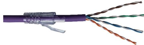
3. Untwist the pairs and straighten the individual wires.
