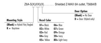
Outlet terminates S/FTP, F/FTP and F/UTP cable constructions with 22 - 26 AWG (0.64 - 0.51mm) solid and 26 AWG (0.48mm) stranded conductors, with up to 0.60mm diameter conductors and up to 1.48mm diameter over insulation.
