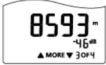
The receive fiber adds 130 m to the length measurement.
