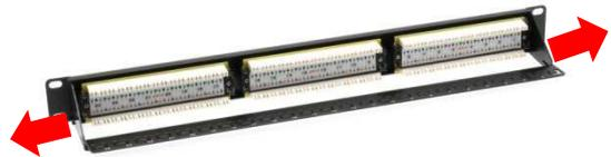
3. Dress the wires in to the appropriate coloured IDC slots following the preferred wiring configuration. Ensure that the cable pair twists are maintained as close as possible to the point of termination.
