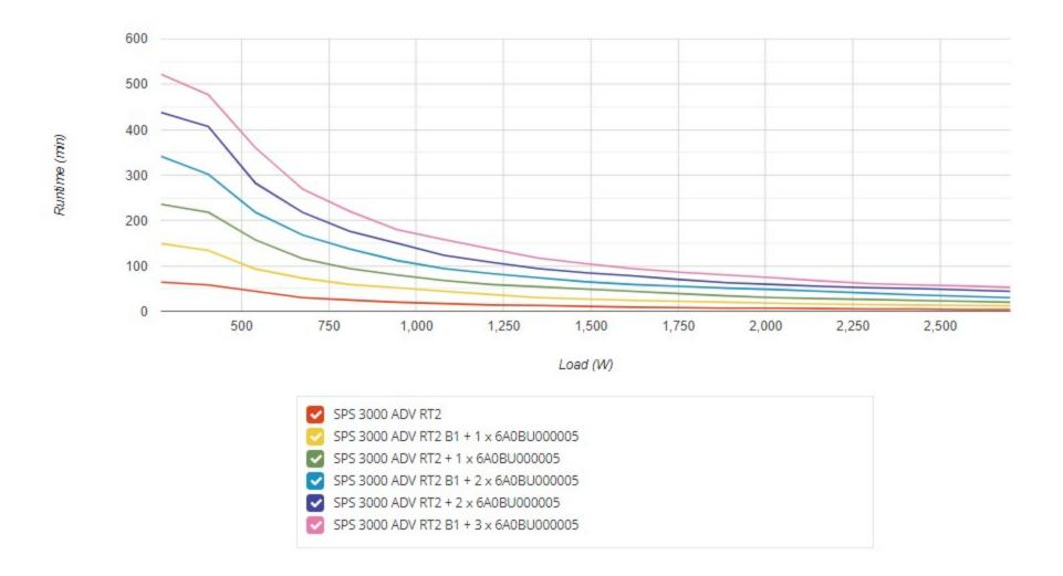
Battery runtimes data: All measurements taken with new, fully charged batteries, at typical environmental conditions, and resistive load (PF = 1.0) output. These figures can differ +/- 15% around these typical values.
