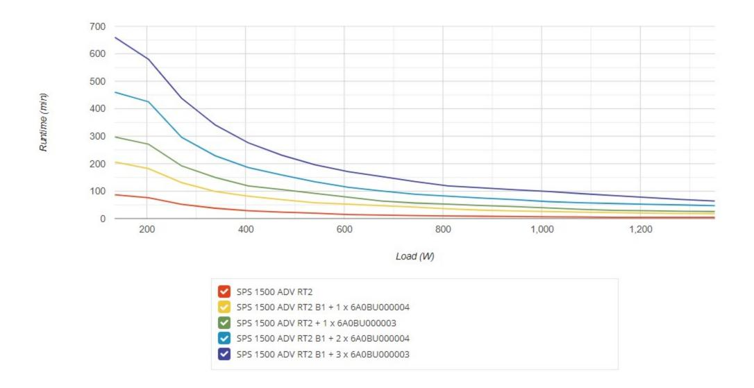
Battery runtimes data: All measurements taken with new, fully charged batteries, at typical environmental conditions, and resistive load (PF = 1.0) output. These figures can differ +/- 15% around these typical values.
