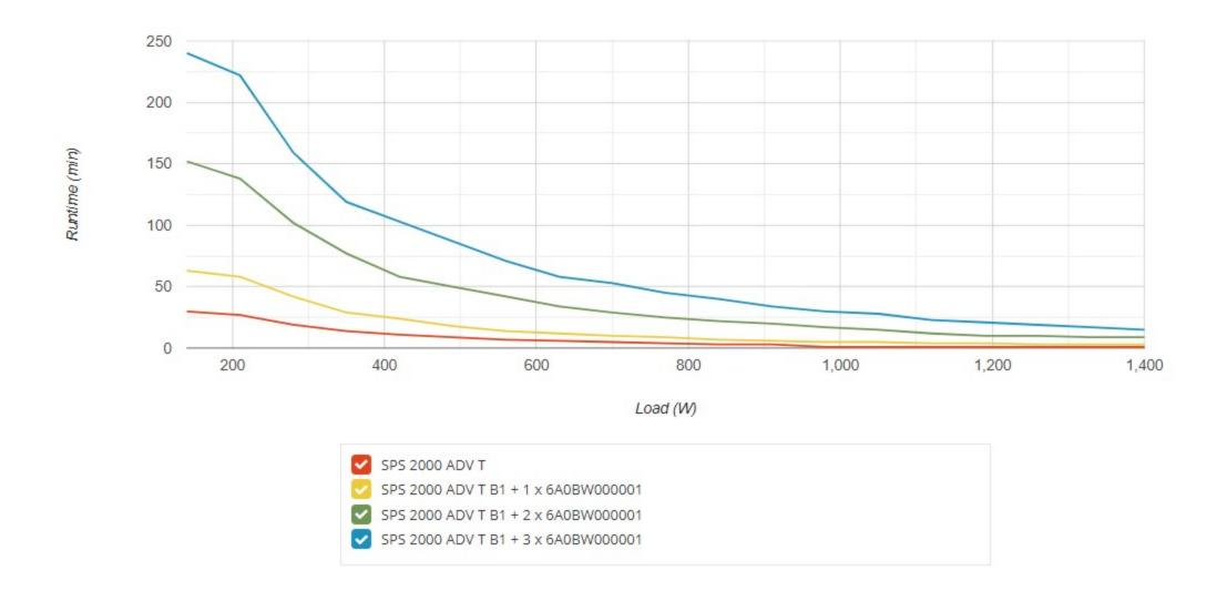
Battery runtimes data: All measurements taken with new, fully charged batteries, at typical environmental conditions, and resistive load (PF = 1.0) output. These figures can differ +/- 15% around these typical values.
