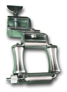
The cable roller guide can be clamped without tools to beams, trays or racks. Also, by removing the clamp part, it can be bolted directly down to unistrut or trays. Fitted with a hinged gate and knurled nut, cable can easily be inserted and removed. The cable roller guide is suitable for cables up to 60mm diameter with a weight capacity of 100Kg
